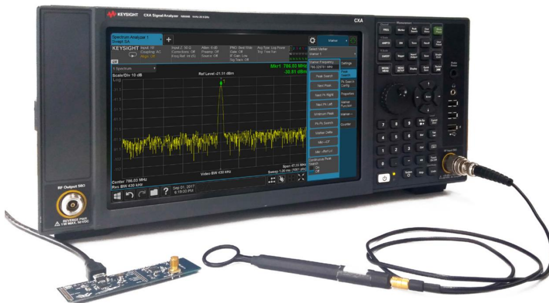
Figure 2: Near-field probe and CXA signal analyzer test the emission of PC LAN port during design cycle before full compliance testing
